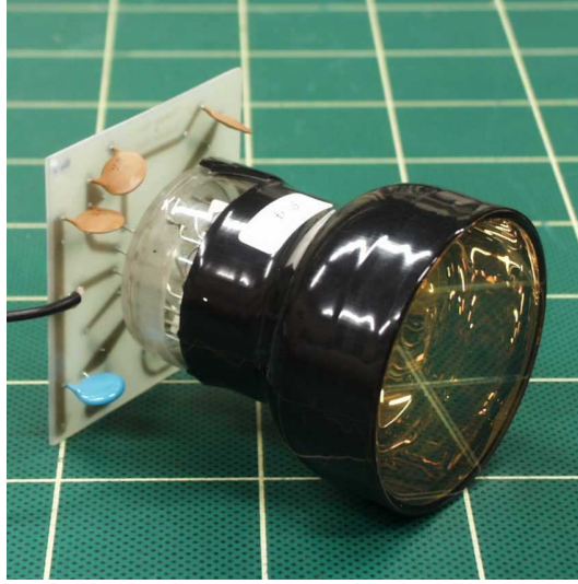
Figure 14: A photograph of a PMT with the PMT base.
