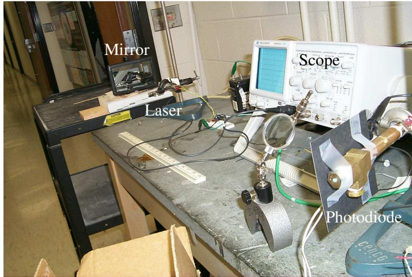
Figure 1: Picture of the set up. You'll notice a different kind of scope in the picture, but otherwise your set-up will be pretty similar.
