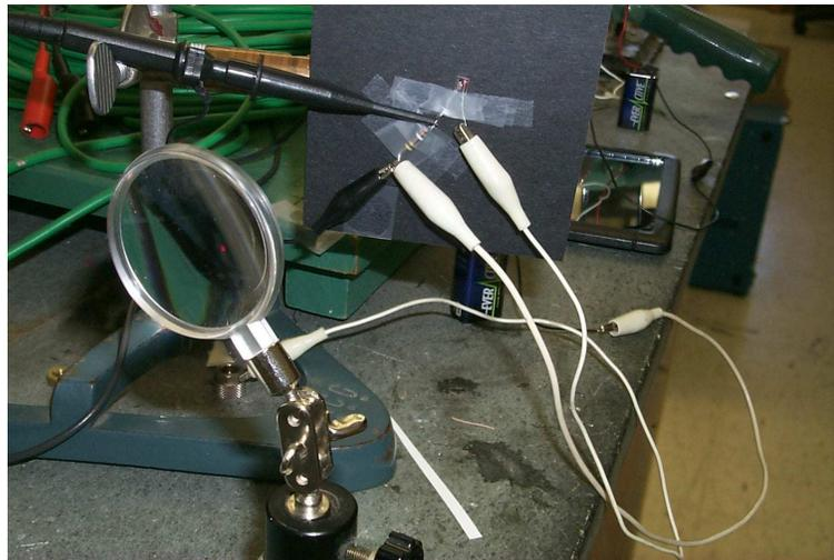
Figure 5: Picture of the photo-diode hook up. Notice the magnifying glass. This can really help to get the laser to be concentrated on the little button of the photo-diode. If you look closely in a color reproduction, you can see a little red dot on the photo-diode and on the lens. That's the laser beam!.
