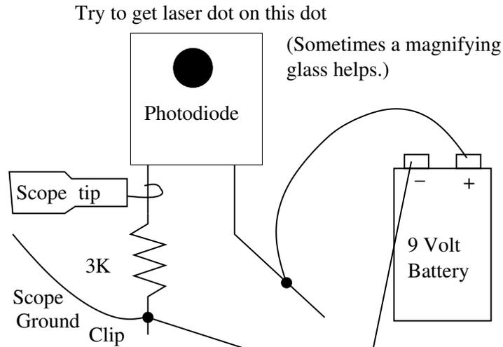
Figure 4: Diagram of the photo-diode hook up.
