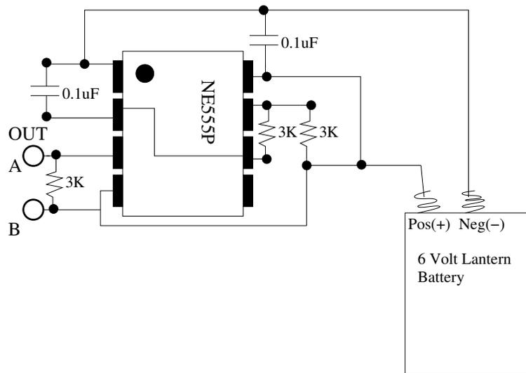
Figure 2: Here is the relevant circuit diagram for the pulser.
